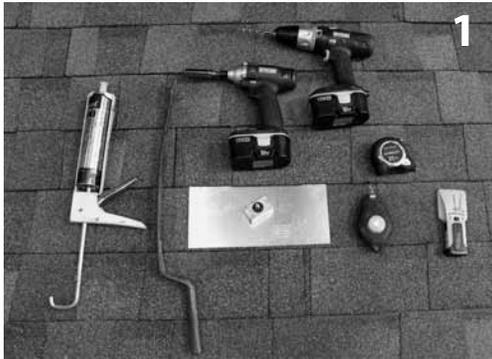
1 Locate, choose, and mark centers of rafters to be mounted. Select each row course of roofing for Mount placement of Quick Mounts.
